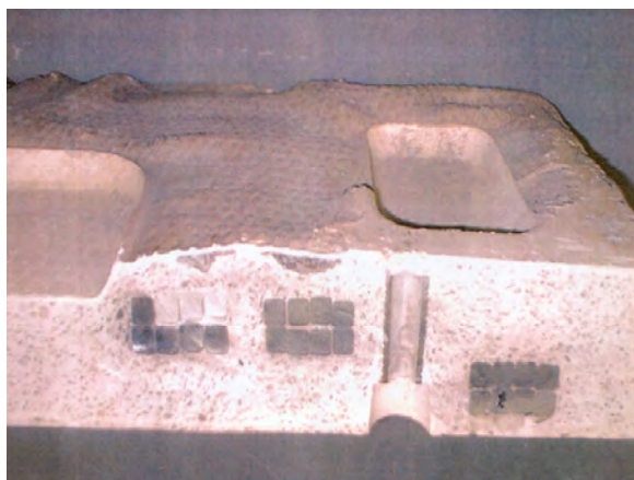
Figure 15 Guideway Loop Panel Enclosed in Polymer Concrete Matrix
