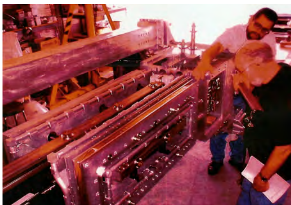
Figure 9 Assembly of Maglev-2000 Superconducting Quadrupole
