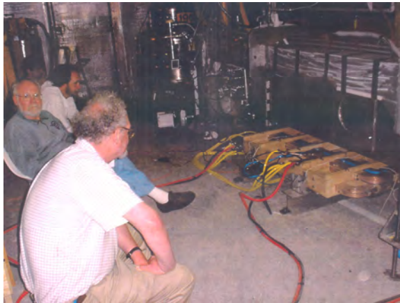
Figure 11 Testing of Magnetic Forces on Maglev-2000 Quadrupole Using DC Current in Aluminum Loop Panel
