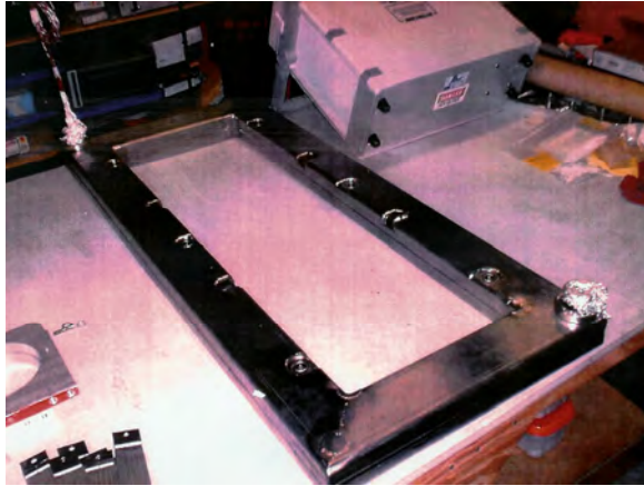
Figure 7 NbTi Superconducting Loop Enclosed in Stainless Steel Jacket
