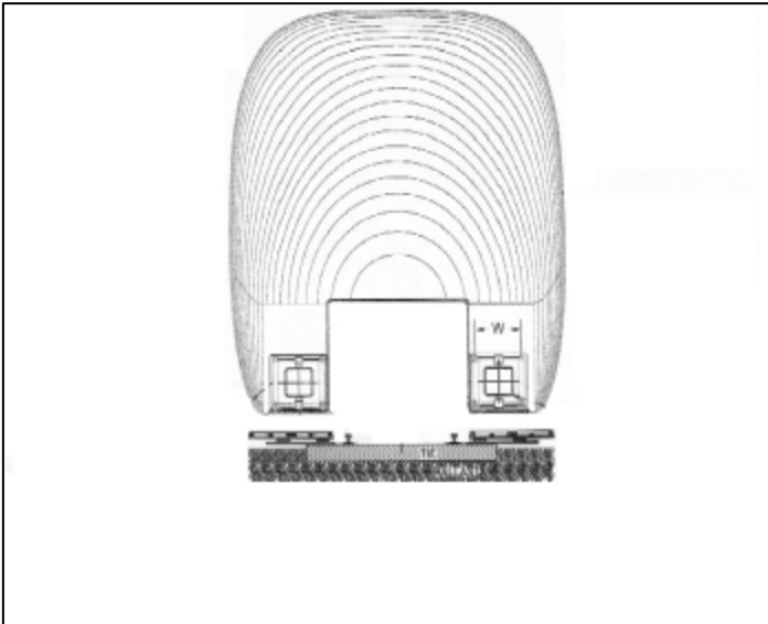
Figure 12. Drawing of levitated Maglev-2000 vehicle traveling on conventional RR track to which aluminum loop panels have been attached to the cross-ties.
