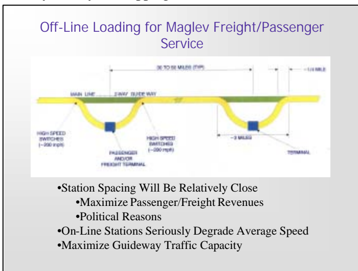
Figure 7. High Speed Electronic Switching of Maglev-2000 Vehicles From Main Guideway to Off-Line Stops
